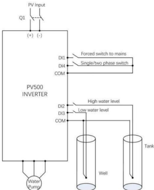
Figure 3-3 Standard wiring diagram
