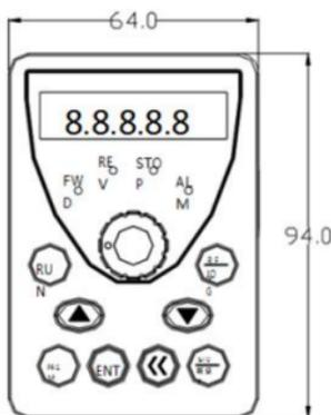
Figure 4-1 Keypad diagram for inverters
